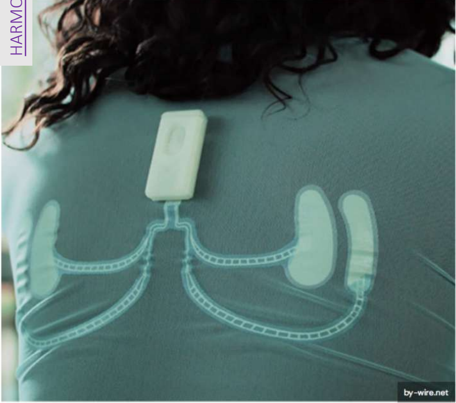
Netherlands-based initiative Closed Loop Smart Athleisure Fashion integrates laminated sensors into clothing that track wellbeing and stress levels
